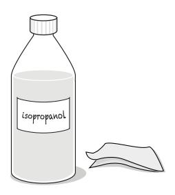
Clean the glass from any dirt, dust or grease using isopropanol or ethanol, then leave to dry.
