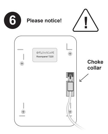
Slip the choke collar of the included cable into the cable pocket. (The choke is needed to eliminate electromagnetic interference)
