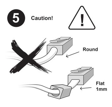
Always use the <u>included</u> ULTRA THIN 1MM Flat cable. Standard round ethernet cable will cause interference!
