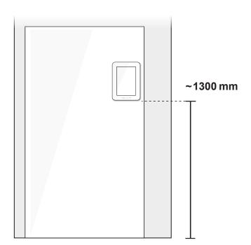
Preferably mount the roompanel close to the window edge to minimize visible cable routing. The cable can be routed in any direction.
