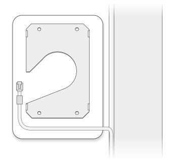
The ultra thin 1mm cable can be slided and hidden in between the plate and the roompanel.
