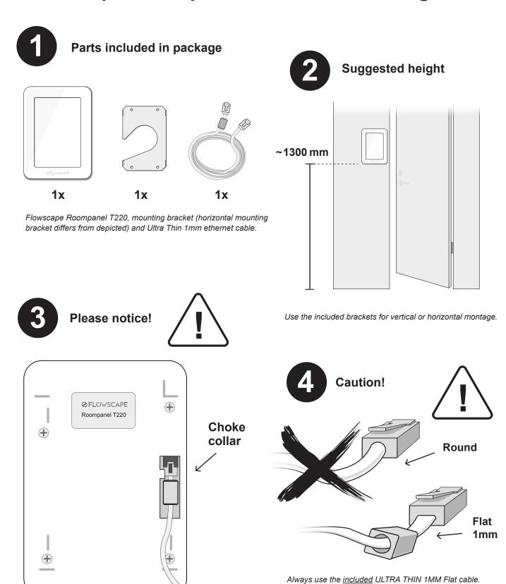
Slip the choke collar of the included cable into the cable pocket. (The choke is needed to eliminate electromagnetic interference)
