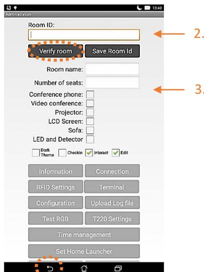
7. When the room panel has been connected to the server and the room id verified press back and wait 10 seconds until the room panel complete the synchronize.
