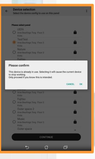
NOTE: If the panel shows a lock icon it is already a Room panel connected to the device. If you click "OK" the old room panel will stop working and be replaced with the new one.
